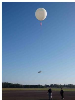
Figure 3: Photo of a Sounding Balloon as an example of the one used within the HEMERA programme.
