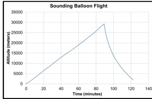
Figure 4: The plot shows the altitude in km of the Sounding Balloon used within the HEMERA programme as a function of the flight time in hours.
