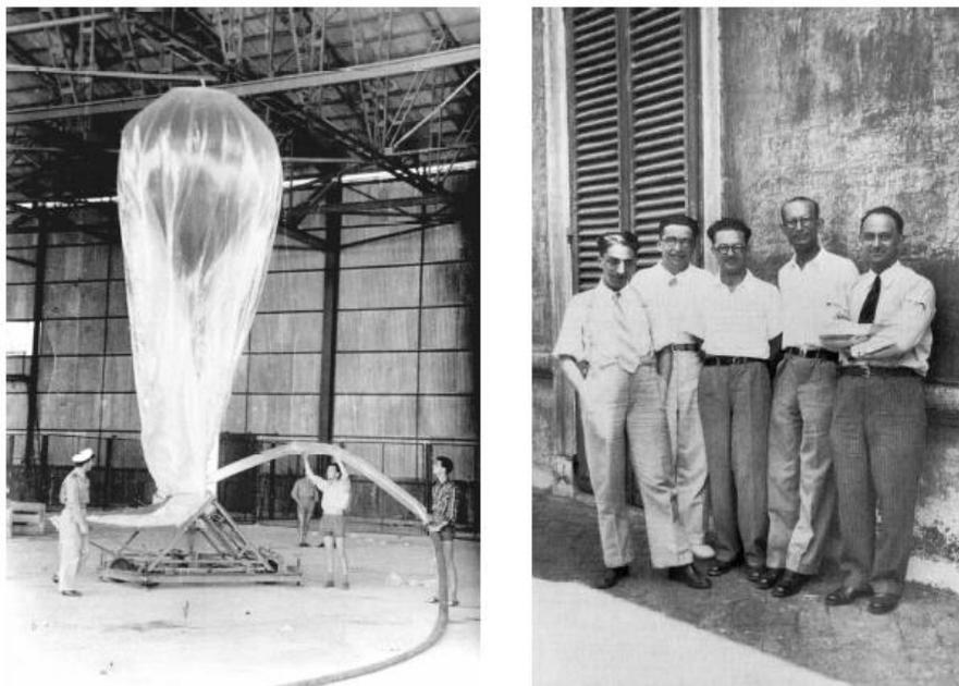
Figure 1: Left: one of the first experiment carried out with stratospheric balloon in Italy is shown. The balloon, with a volume of about 9,000 cubic meters, was launched from the Cagliari Elmas Airport (Sardinia, Italy).The experiment was designed and exploited under the lead of Prof. Edoardo Amaldi. Right: The group of the "Ragazzi di Via Panisperna": starting from the left: Oscar D'Agostino, Emilio Segre, Edoardo Amaldi, Franco Rasetti ed Enrico Fermi.
