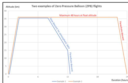
Figure 6: The plot shows the altitude in km of the Zero Pressure Balloon used within the HEMERA programme as a function of the flight time in hours.
