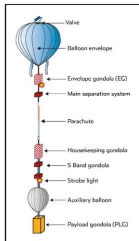
Figure 5: Scheme of a Zero Pressure Balloon used within the HEMERA programme.
