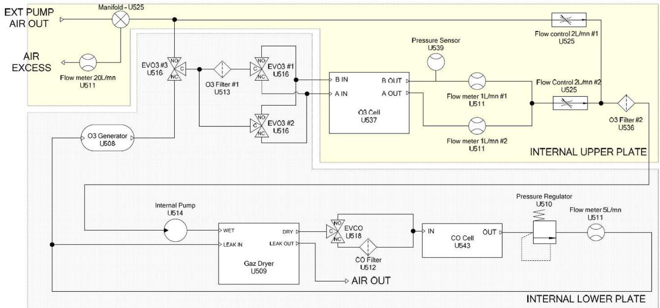
Figure 6: Flow diagram of IAGOS Package1, showing all pneumatic connections for O3 and CO measurements.
