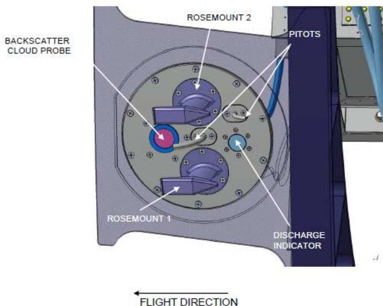
**Figure 4** : IAGOS Inlet plate : Forward facing pitot for Package1 air, backward pitot for Package2 exhaust. Rosemount 1 holds the H<sub>2</sub>O sensor, Rosemount2 holds the Package2 inlet.
