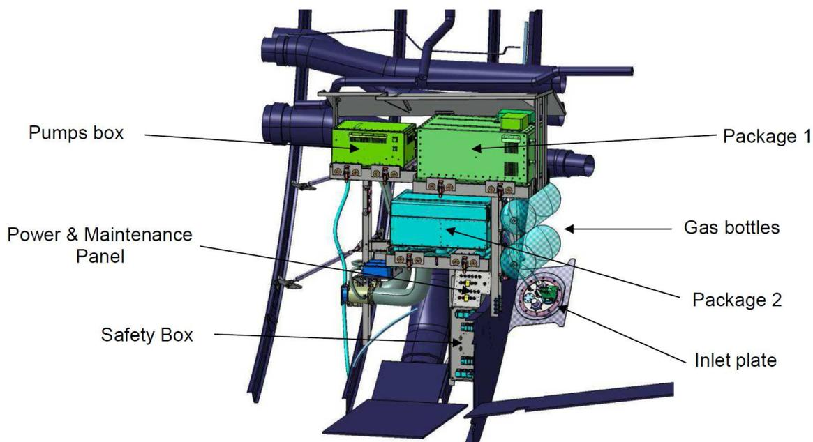
**Figure 1:** IAGOS installation aboard Airbus aircraft
