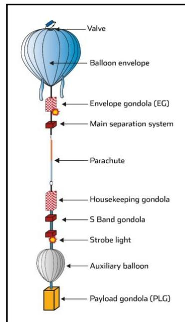
Fig. 4: Scheme of a Zero Pressure Balloon provided by the HEMERA programme
