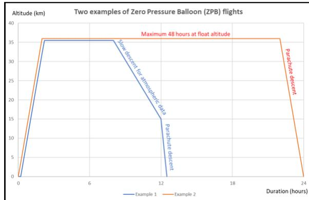
Fig. 5: The plot shows the altitude reached by the ZPB as a function of the time of flight.
