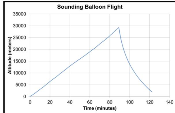
Fig. 3: The plot shows the altitude in meters as a function of time in minutes of the SB provided by the HEMERA programme.
